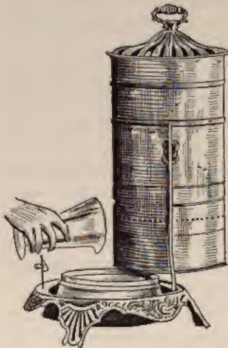
FIG. 248.—Kuhn formaldehyde generator. Filling. (Rosenau.)
